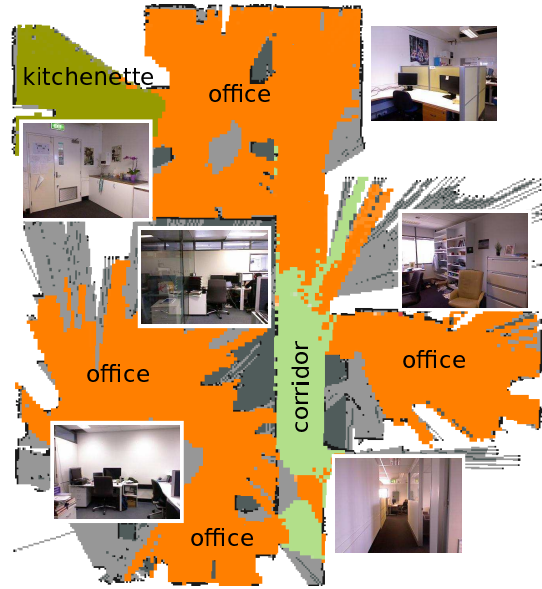
Fig. 5: A semantic map generated by a combination of laser-based gmapping and a vision-based scene classifier using the Places205 ConvNet. The colors encode the semantic categories of different places encountered in the environment. The figure shows a map of an office environment (orange) with a kitchenette (dark green) and a long corridor (light green).
